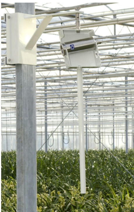
Plant temperature camera placed in a suspension bracket.
