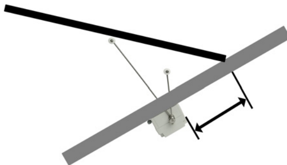
Vent position indicator fitted
